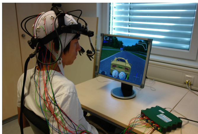
Figure 1. A participant testing the novel bi-modal interface. EEG and eye gaze data are acquired and processed on-line for controlling the driving simulator.
