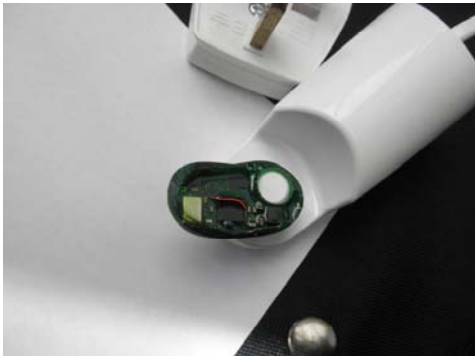
Figure 3, An OPTIMI sensor in encapsulation and on inductive charge.
