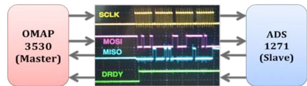
Figure 5: The SPI communication between OMAP3 and the ADC
